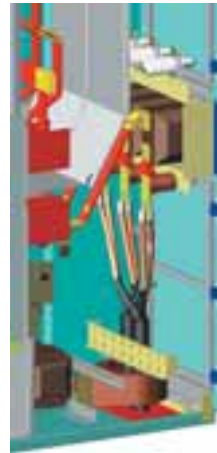
Power cable entry (example)
