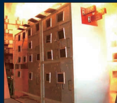
Arcing due to internal fault tested 内部アーク短絡試験
